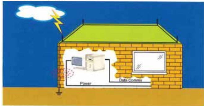
Inductive coupling from a lightning conductor
